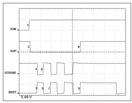
Figure 15: Three-Byte Response Packet Read from the SKB Switch
