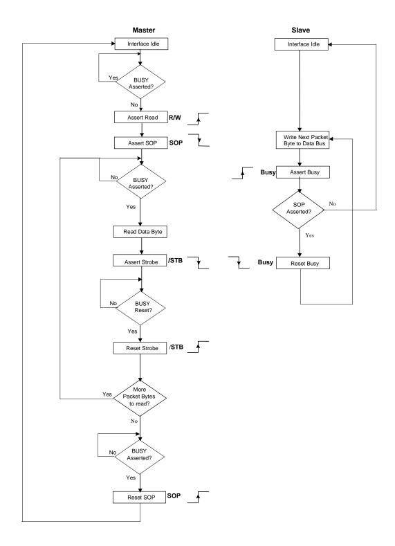
Figure 13: Flowchart of Read Cycle
