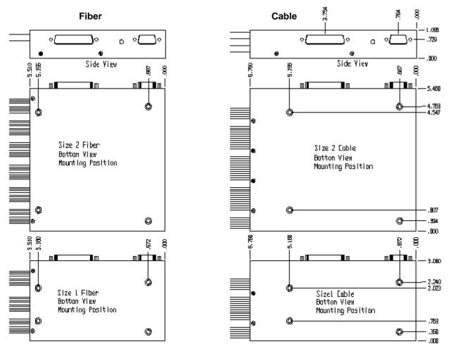
Figure 6: Mounting Hole Locations for Fiber and Cable Versions
