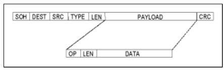
Figure 9: RS485 Link-Layer Packet and Command Packet
