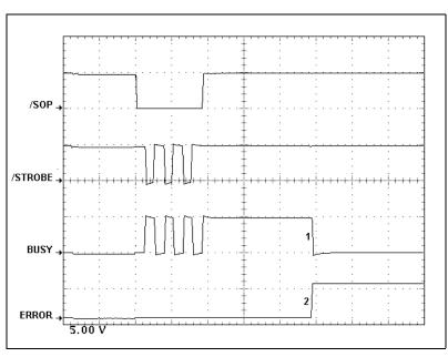
Figure 17: Three-Byte Packet Write Produces an Error
