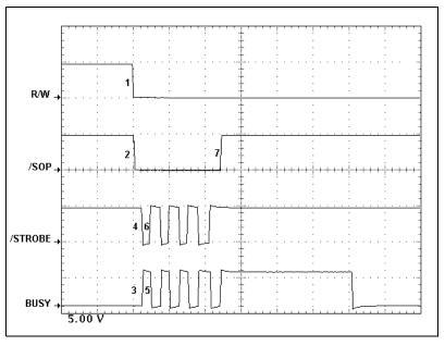
Figure 16: Four-Byte Command Packet Write to the SKB Switch
