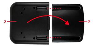
3. Slide the Seeker MCA III (3) forward until the Alignment Tab (4) comes into contact with the back side of the mobile mount (2).
