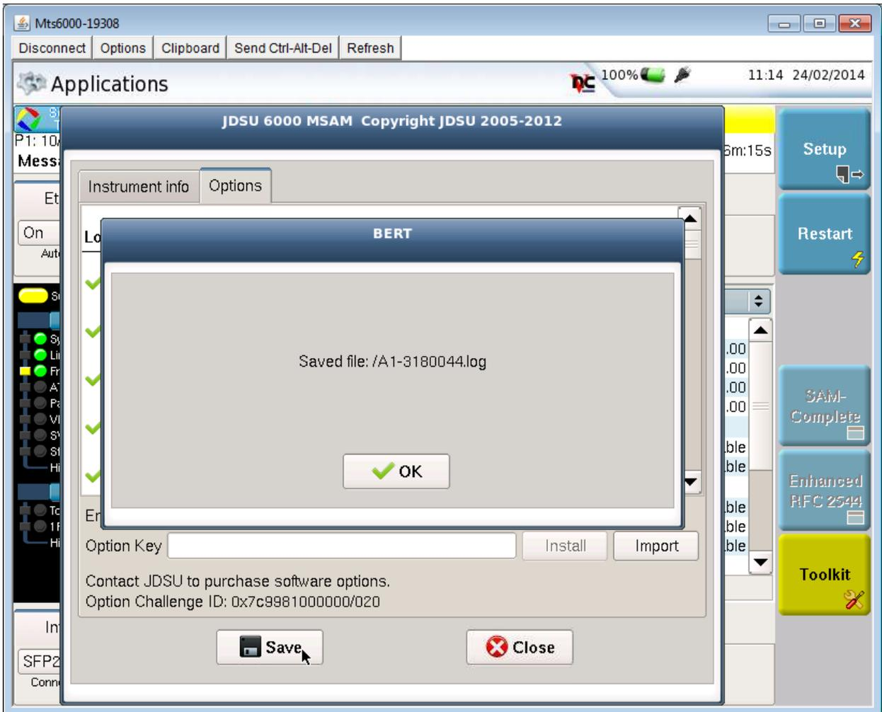
**To retrieve the log file press FILE and the Click on the bert folder. The log file can then be copied to a USB stick and emailed by selectin the log file and the pressing EDIT and then COPY. To paste it to the USB device touch on the USB entry in the directory listing on the left to select the USB and then press EDIT and PASTE.**
