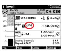
Equalizer warning appears in the signal measurement screen indicating an equalizer-related issue
