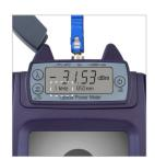
The power meter detects light signals modulated at standard frequencies of 270Hz, 330Hz, 1kHz, and 2kHz. If one of these frequencies is detected, it appears in the display.
