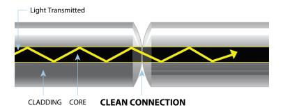
Today's connector design and production techniques have eliminated most of the challenges to achieving **core alignment** and **physical contact.** What remains challenging is maintaining a **pristine end face.**
