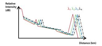
Figure 28: Multi-wavelength OTDR traces of a Pulse Delay method
