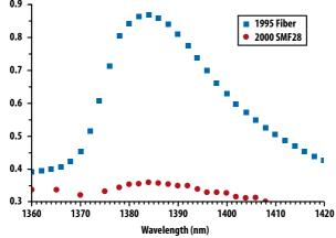
Figure 62: OH- absorption vs. fiber manufacturing time
