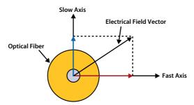
Figure 36: Signals transmitted through a birefringent fiber experience a slow and fast polarization mode
