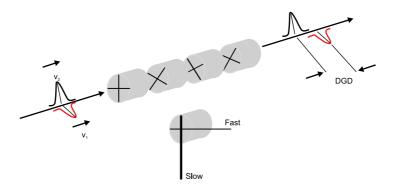
Figure 39: Strong mode coupling in telecommunications optical fiber
