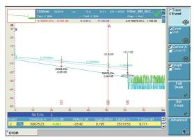
Figure 82: Multi-wavelength OTDR measurement with the JDSU OTDR module range
