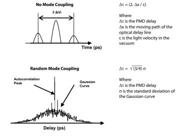
Figure 55: Interferometry response according to type of mode coupling
