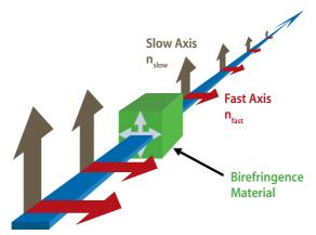
Figure 33: Propagation in a birefringence material
