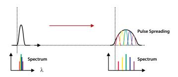
Figure 1: Pulse spreading caused by wavelengths traveling at different group velocities
