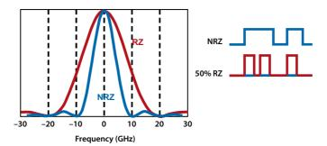
Figure 16: Optical bandwidth of a NRZ and 50 percent RZ amplitude modulated signal (both operating at the same data rate)
