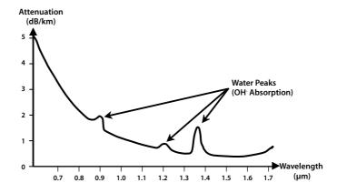
Figure 59: Fiber attenuation as a function of wavelength
