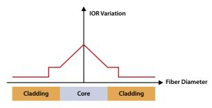
Figure 11: Schematic of index of refraction variation for an NZ-DSF
