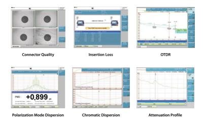
Figure 90: Summary of link characterization tests
