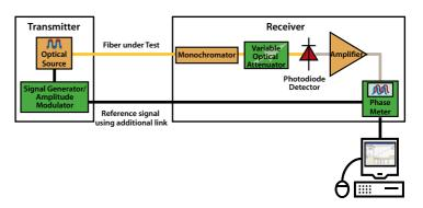
Figure 24: Typical schematic of the elements of the Phase Shift method
