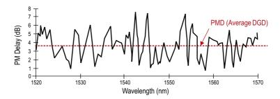
Figure 40: DGD as a function of optical wavelength
