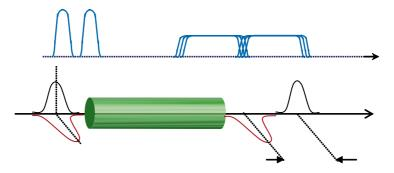
Figure 42: Typical signal distortions caused by excessive PMD in a fiber transmission line
