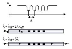
Figure 22: Schematic of a fiber Bragg grating
