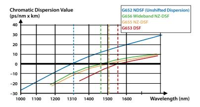
Figure 12: Dispersion curves according to fiber types
