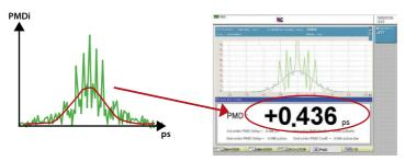
Figure 87: PMD measurement display with the JDSU Fixed Analyzer method in the T-BERD/MTS platform
