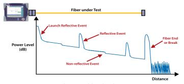
Figure 81:T-BERD/MTS-8000 with OTDR module and resulting trace
