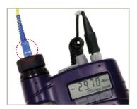
Figure 71: Patch cord inspection
