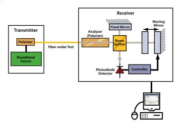
Figure 56: Typical schematic of the elements of the TINTY method
