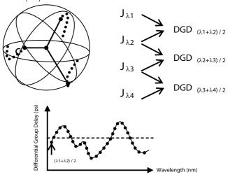
The accuracy at which the DGD can be determined increases with the frequency range within which the Jones matrix is analyzed. The frequency steps for the tunable laser have to be chosen carefully to match the expected DGD in the fiber.
