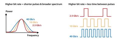
Figure 15: Effect of bit rate increase on pulse width and intervals
