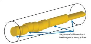
Figure 38: Fiber birefringence in an optical fiber link
