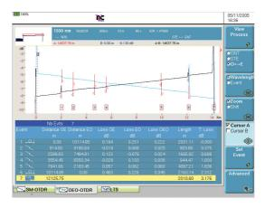
Figure 83: Bidirectional OTDR analysis with the JDSU T-BERD/MTS platforms
