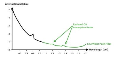
Figure 60: Fiber attenuation as a function of wavelength
