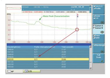
Figure 65: Measuring the attenuation profile with the T-BERD/MTS-8000
