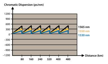
Figure 20: Difference between no slope management and slope management for three wavelengths being compensated with the same magnitude
