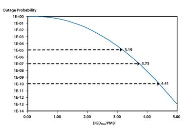
Figure 43: Outage probability vs DGD<sub>Max</sub>/PMD
