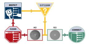
Figure 70: Connector inspection and cleaning steps
