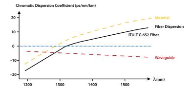
Figure 8: Total CD of a single-mode fiber = material + waveguide dispersion
