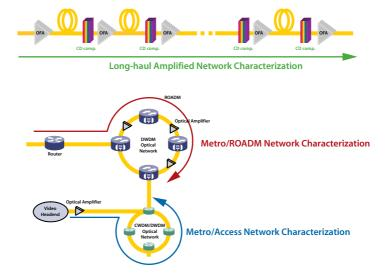
Figure 66: Example of route of tests for network characterization
