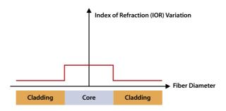
Figure 9: Schematic of index of refraction variation for an SSMF
