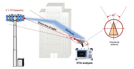
Figure 22. Multipath effect in OTA measurements
