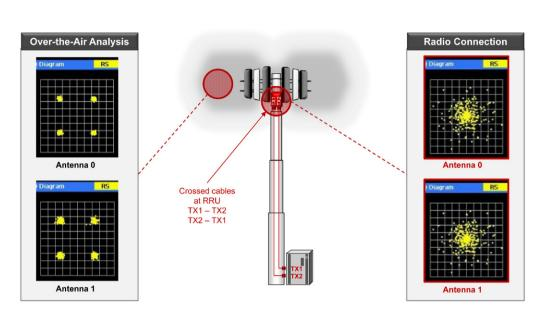
Figure 20. MIMO failure due to cross cabling
