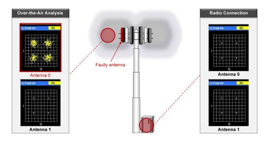
Figure 19. MIMO failure due to antenna 0
