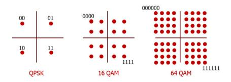
Figure 6. User data (PDSCH) modulation types
