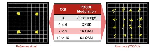
Figure 9. Reference signal and user data (16 QAM)
