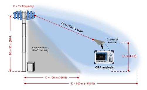
Figure 23. Path loss effects in OTA measurements
