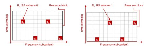
Figure 15. Cell-specific RS for antennas 0 and 1 in an RB
