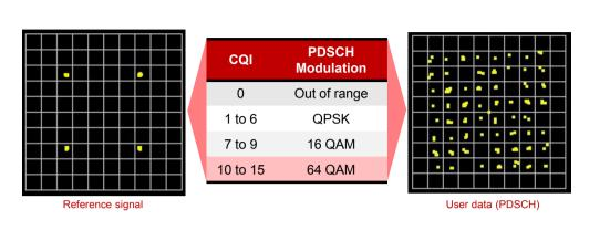
Figure 10. Reference signal and user data (64 QAM)
