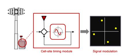
Figure 12. Cell site in free run
