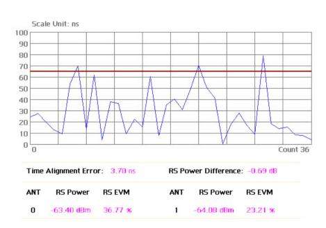
Figure 18. MIMO time alignment error antenna 0 (RS0) and antenna 1 (RS1)
