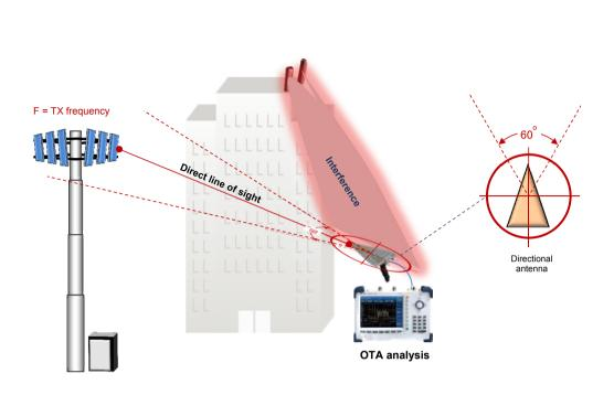
Figure 21. Interference effects in OTA measurements
