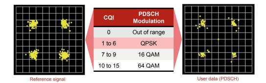
Figure 8. Reference signal and user data (QPSK)
