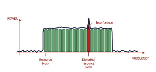
Figure 2. LTE signal distorted by interference
