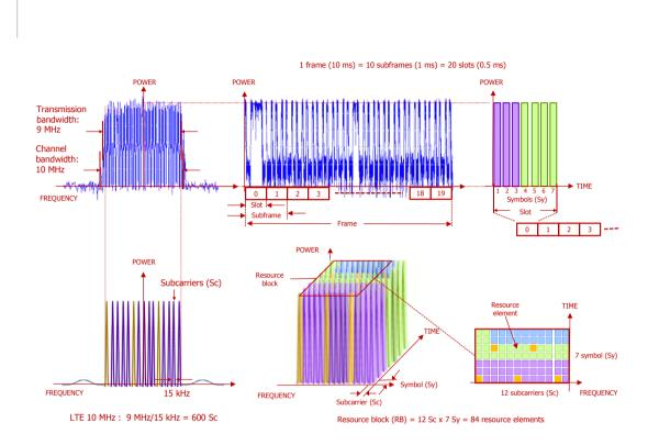
Figure 1. LTE signal format
