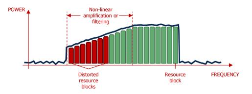
Figure 3. LTE signal distorted by non-linear amplification or filtering
