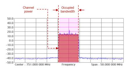
Figure 4. LTE channel power and occupied bandwidth
