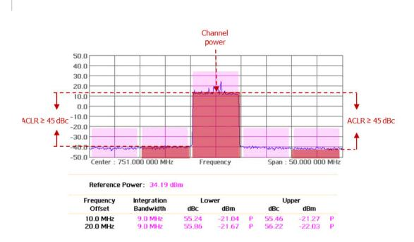
Figure 5. LTE adjacent channel leakage power ratio
