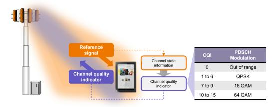
Figure 7. RF environment assessment (via reference signals) and CQI
