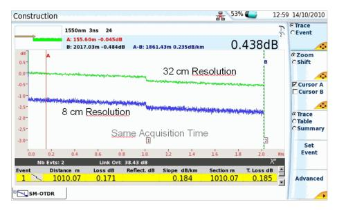
Figure 2. High resolution requires more acquisition time to achieve optimized trace
