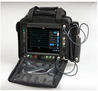
The 8800SX in Soft Case with Return Loss Bridge Connected
