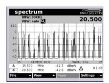
The Ingress Expert FFT captures the whole noise envelope at once, and there's no need to wait for multiple scans to see complete interference impact, or recognize the signature of the interfering signal.
