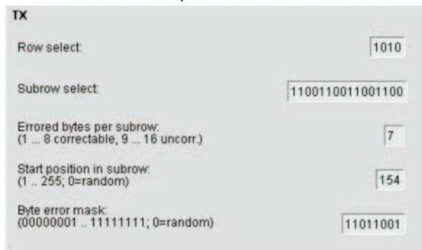
Figure 6: Parameters for specification in FEC\_adv feature
