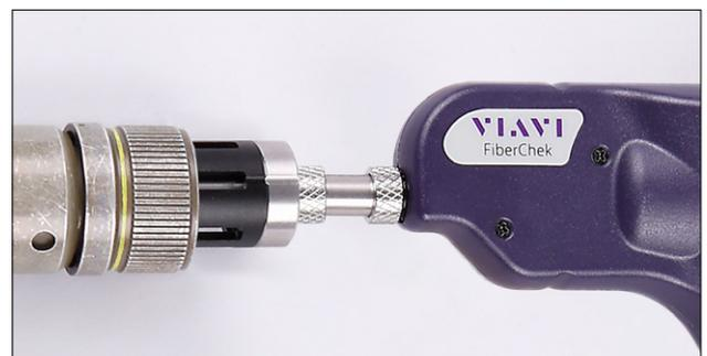
The new MIL-PRF-28876 plug and receptacle inspection guides are listed below. All these guides use a FBPP-BAP1-G barrel assembly compatible with P5000i and FiberChek probe microscopes.
