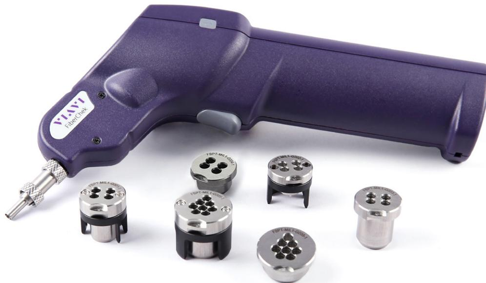
MIL-PRF-28876 fiber optic connectors are environmentally hardened for harsh environments such as shipboard use cases. The VI·AVI MIL-PRF-28876 inspection guides are used with P5000i USB probe microscopes and FiberChek all-in-one handheld probe microscopes for visual and automated assessment of fiber optic termini end faces. It is essential to inspect before connecting fiber optic connectors to ensure that the end face is sufficiently defect-free to be put into service.
