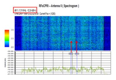
Comparative spectrogram results showing consistent interference on both antennas; note rolling rises in the noise floor across the whole band
