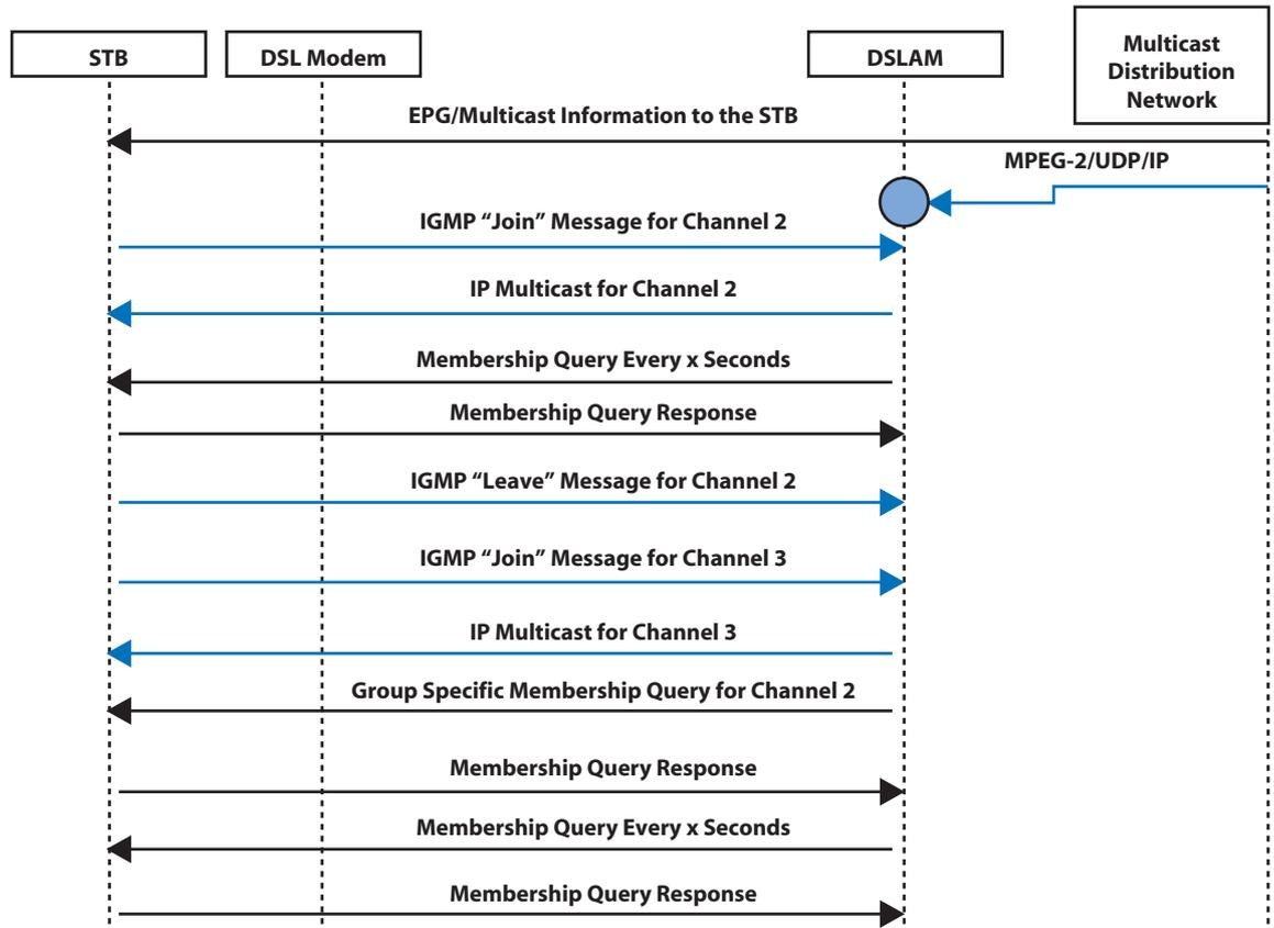
Figure 2. An example of an IGMP message flow
