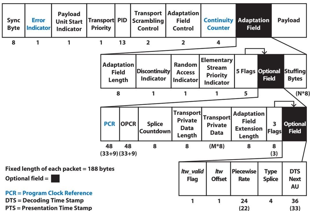
Figure 1. A schematic diagram of the transport stream packet header
