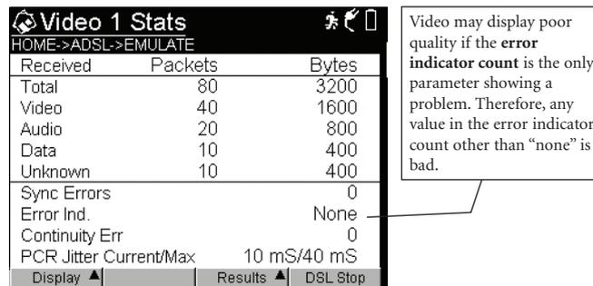
Figure 4. Packet statistics for video, audio, and data portions of the stream
