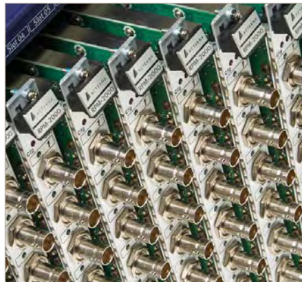
Close-up view of the rear of an HCU1500 showing RPM2000 modules.
