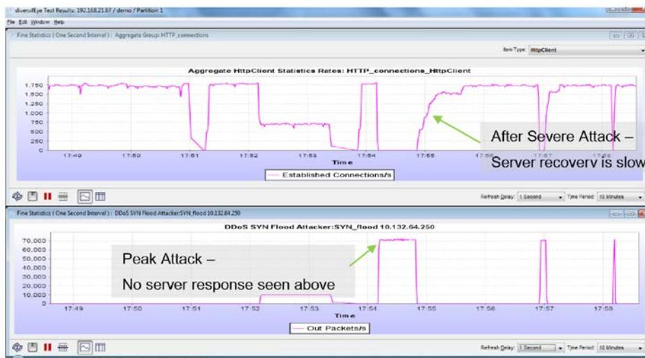
Figure 2 : The impact of a DDoS type attack in a secure VPN connection.
