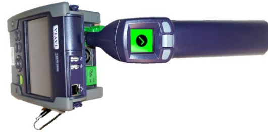
Figure 3: OTDR Port Inspection
