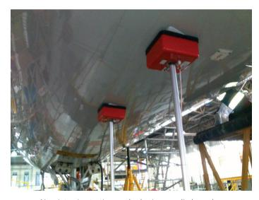
Non-intrusive testing method using supplied couplers simulates flight conditions
