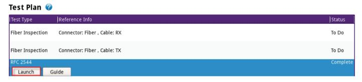
The test set automatically configures to the test to be conducted (in this example, RFC 2544), conducts the test according to a configuration file, and executes the test to completion.
