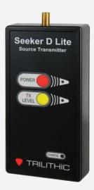
Both devices provide an uncompromising tagging solution for active analog or digital systems and can be used to identify and locate all RF leaks in both the Aeronautical and LTE bands.
