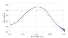
Figure 4: 1550nm SLED Spectral Width
