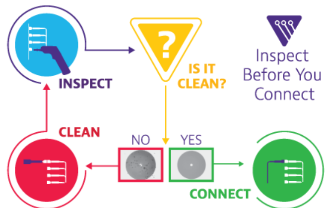
Figure 2: Inspect Before You Connect
