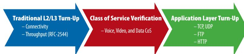
Figure 2: Workflow for Application-Centric Turn-Up
