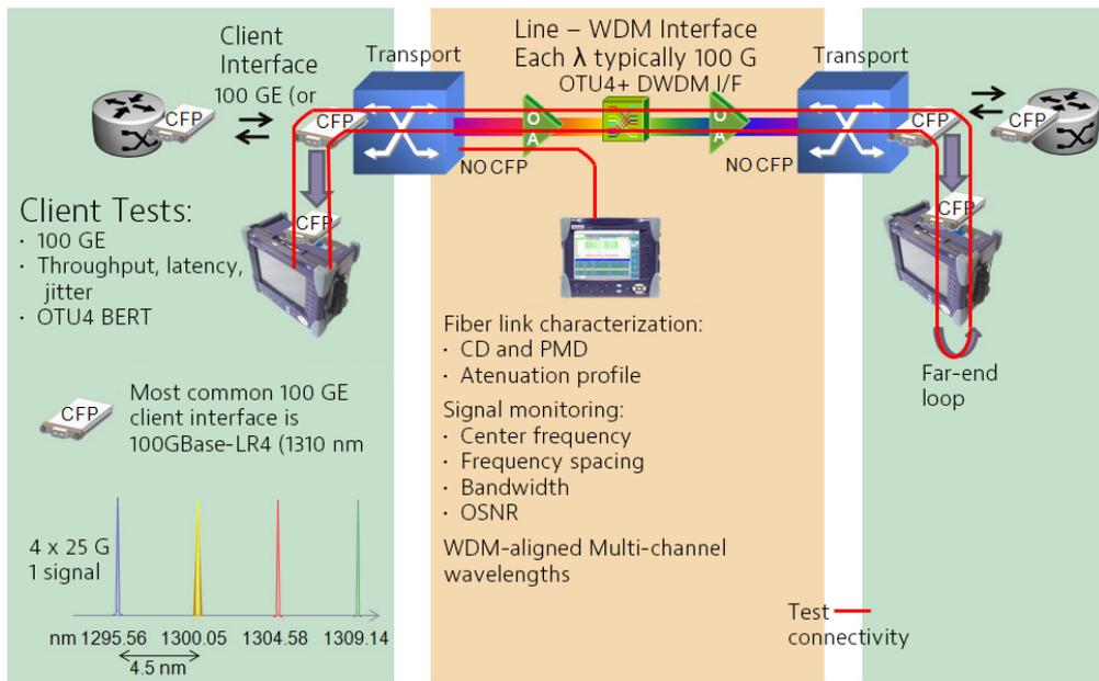
Figure 2. Line and client interfaces
