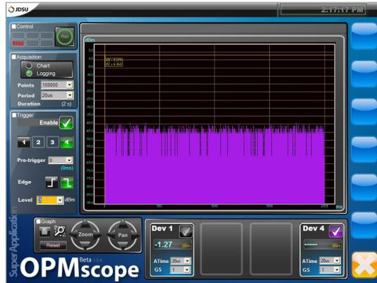
Figure 7: Falling edge triggered logging
