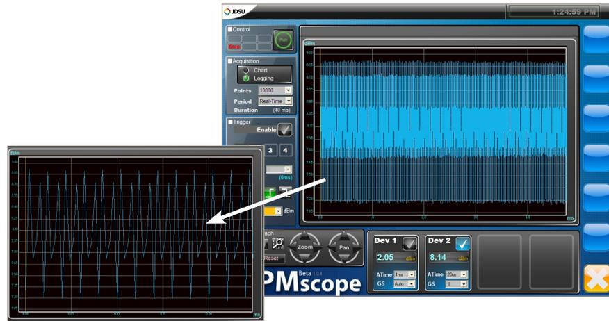
Figure 2a: Optical signal sampled at 4  $\mu$ s
