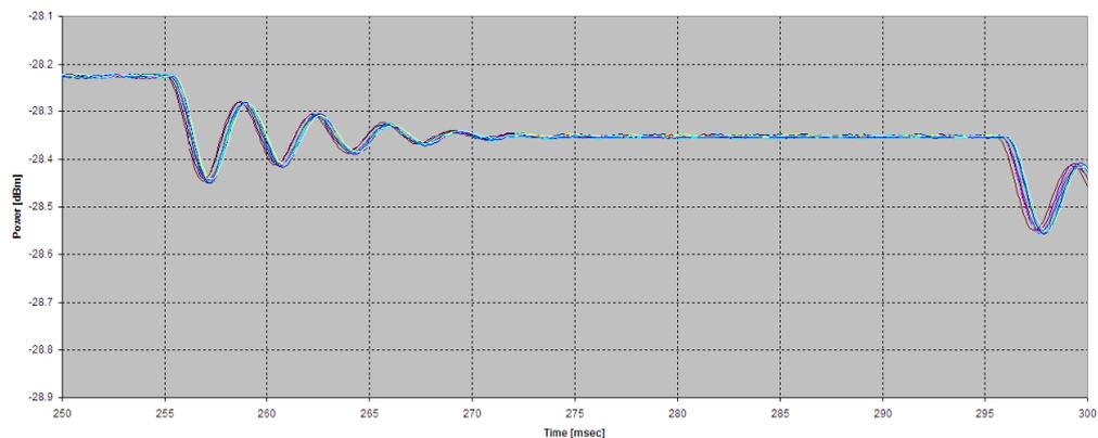
Figure 1: Measuring settling time in the optical domain
