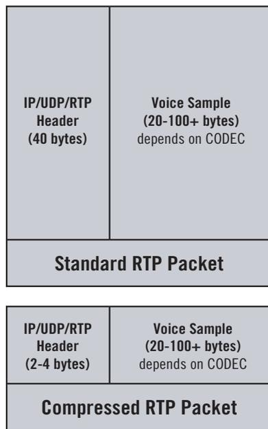
Because the IP header is compressed with the UDP and RTP headers down to a maximum of 4 bytes, leaving no room for an IP address; therefore, the packet cannot be routed. It can only be placed on a point-to-point link that requires no addressing.
