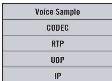
RTP information is encapsulated in a UDP packet. If an RTP packet is lost or dropped by the network, it will not be retransmitted (as is standard for UDP). This is because a user would not want a long pause or delay in the conversation due to the network or the phones requesting lost packets. The network should be designed, though, so that few packets are lost in transmission.
