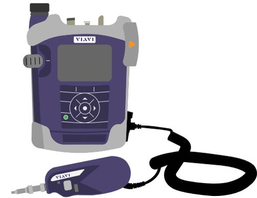
Testing LC-LC configurations that have MPO connections within the links is not different than a typical LC-LC test. As long as the connectors at the end of the link or channel are LC, then the test is the same as other tests performed with LC connections. For a Tier 1 (basic) test, you can use a standard Optical Loss Test Set (OLTS), such as an OLTS-85 that already has native LC ports on the device, so the test cords can be connected directly to the instrument.
